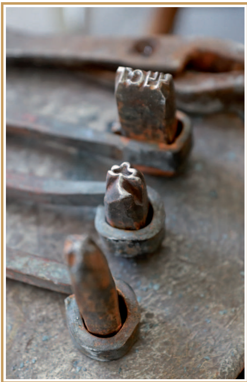
In the process of making a knife, the product is given a traditional beak-shape. Also put on the blade is the corporate seal of Chust with the image of a star.
